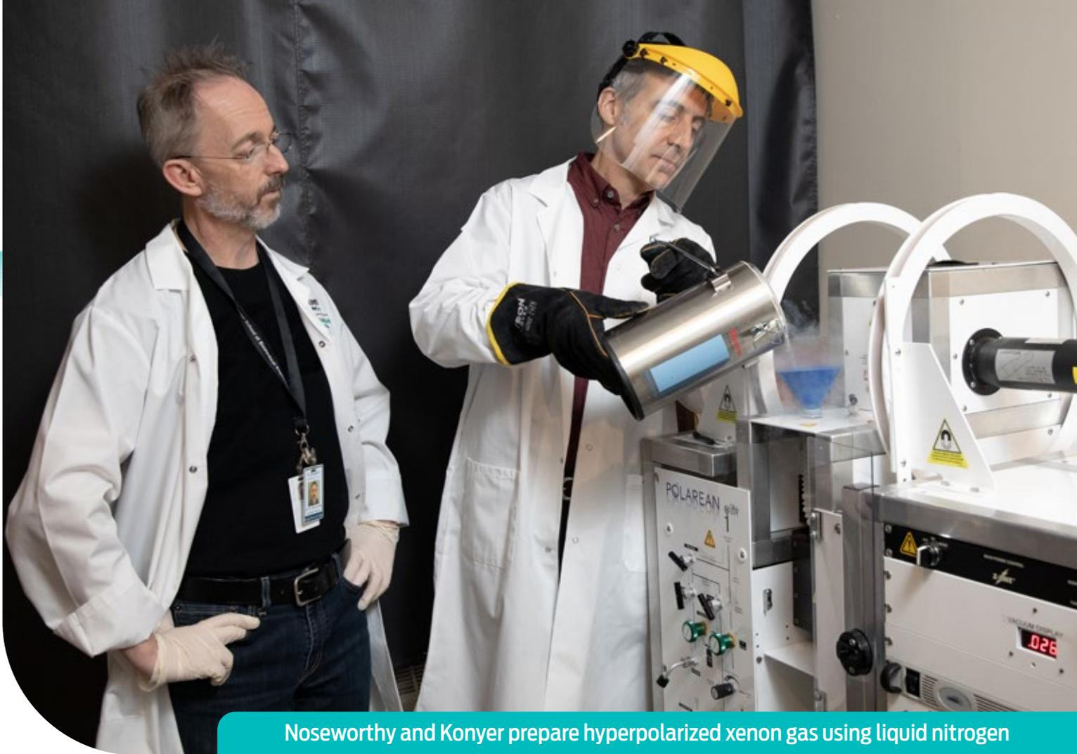
Noseworthy and Konyer prepare hyperpolarized xenon gas using liquid nitrogen
